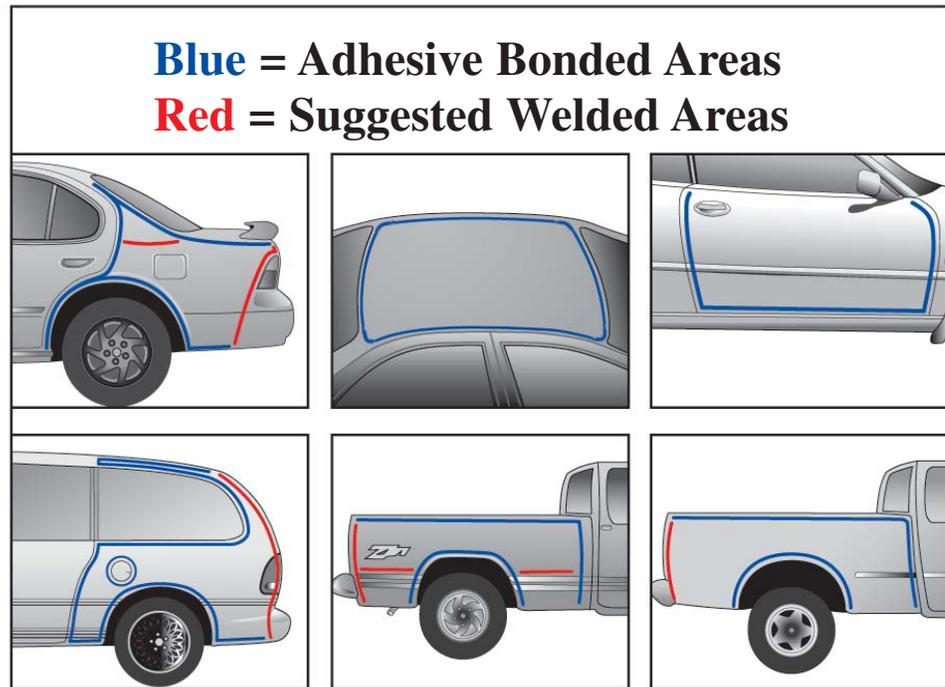
**Caution:** The adhesive is combustible. Keep any MIG welding a minimum of two inches from the adhesive. As with any welding operation, keep the appropriate fire extinguisher within reach, and be alert to any smoke or flame that may be present. Resistance spot welding through uncured adhesive is acceptable.
